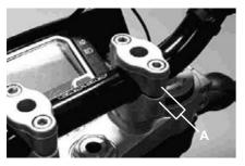
If the handlebar is installed correctly, there will be an even gap at the front and rear after tightening (A).
