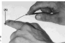
Apply grease inside the gas cable (A).
