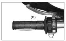
2. After racing the engine slightly, close the throttle completely and depress the engine stop button (D).
