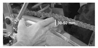
In addition to checking the slack, rotate the rear wheel to inspect for damaged rollers, loose pin and links, unevenly or excessively worn teet, and damaged teeth.
