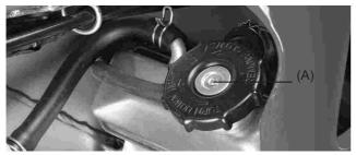
NOTE Check the level when the engine is cold.
