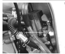
3. If the engine is cold, pull up the choke knob (B).
