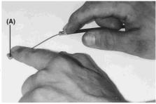
Apply grease to the following point throttle inner cable upper ends.
