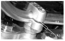
If the handlebar clamp is correctly installed, there will be an even gap at the front and rear after tightening. (A).
