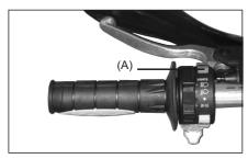
2. After racing the engine slightly, close the throttle completely and push the engine stop button (A).
