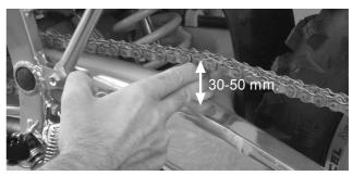
In addition to checking the slack, rotate the rear wheel to inspect the drive chain and sprockets for damaged rollers, loose pin and links, unevenly or excessively worn teet, and damaged teeth.
